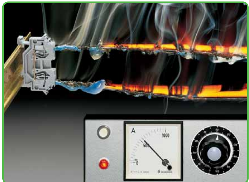
Test arrangement "short time withstand current test"
