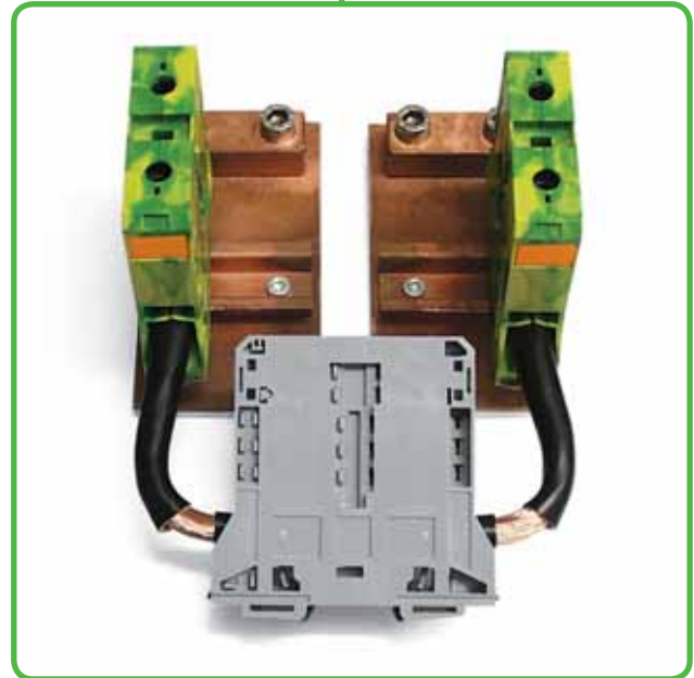
Test arrangement "short time withstand current test"
